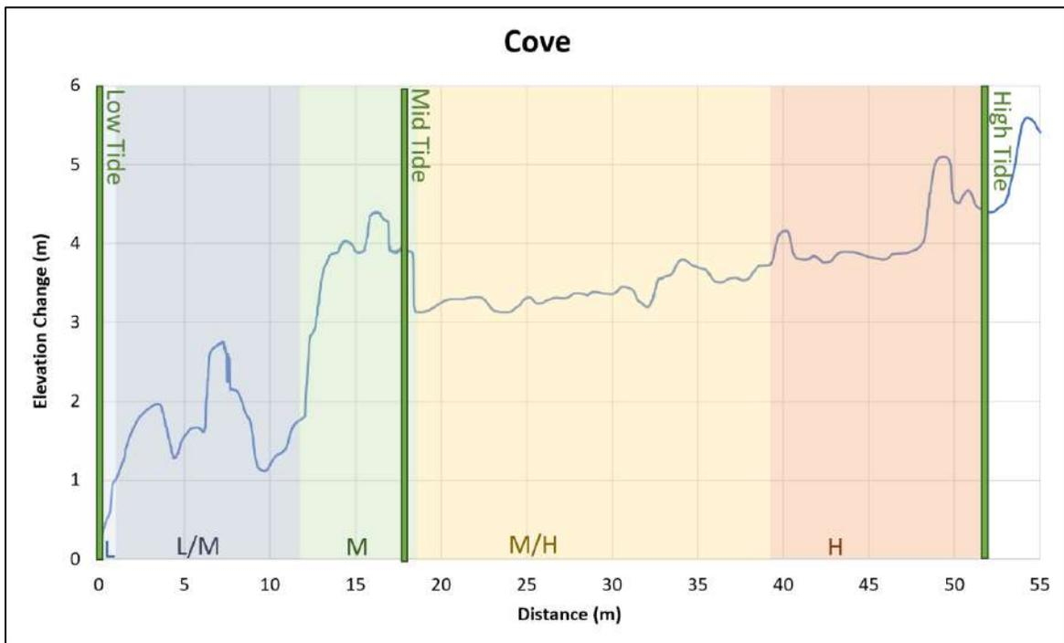
Figure 11. Elevation from Cove site, elevation data was collected through the drone flight that took place on September 27<sup>th</sup>, 2023, through digital elevation models.
