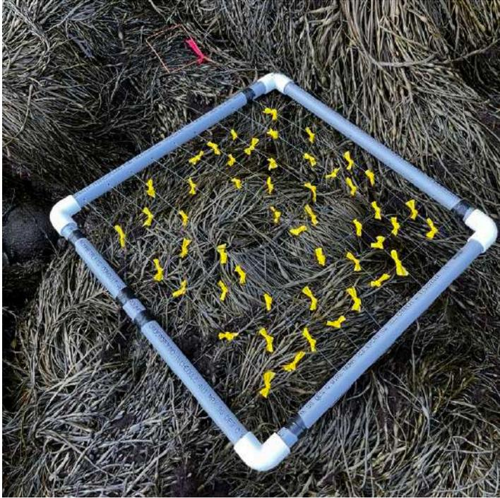
*Figure 8.* Quadrat set up during Cove survey visit on October 27<sup>th</sup>, 2023, showing both the algal cover 50-point random sampling quadrat (0.5m x 0.5m) and the invertebrate abundance quadrat to the upper left (10cm x 10cm).
