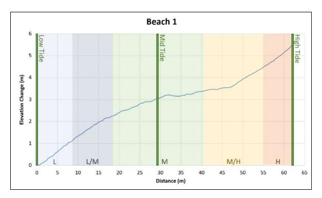
*Figure* 10. Elevation from Beach One site, elevation data was collected through the drone flight that took place on September 27<sup>th</sup>, 2023, through digital elevation models.
