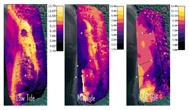
*Figure* 37. Thermal drone imagery of Beach One site, left image shows site at low tide, middle image shows site at mid tide, right image shows site at high tide, all thermal imagery was collected on September 27<sup>th</sup>, 2023.
